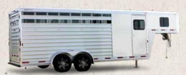
The Express 3H & 4H CX models are the most affordable and convenient models in our gooseneck lineup. These trailers feature all-aluminum construction, a separate dressing room with a saddle rack and tack items, curbside and streetside air gaps, aluminum wheels with radial tires and rubber torsion axles.
