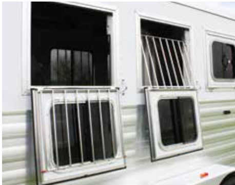
FEED DOORS - Feed doors provide maximum airflow, a rugged look and a durable design
