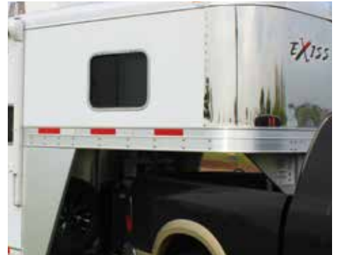
TRAILER NOSE - The large (8' long) Exiss nose allows for more depth and height in the bunk area
